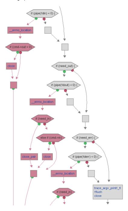
In this logic layout diamond-shaped symbols represent decisions. Blocks of in-line code are contained in rectangles. Unexercised code is shown in red shapes and paths.
